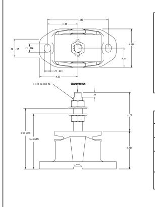
27458 Marine Mounts are compact, captive marine isolators designed to support medium to heavy loads from 350–1,980 lbs. per mount.
