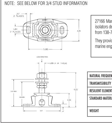
27166 Marine Mounts are compact, captive marine isolators designed to support light to medium loads from 138-750 lbs. per mount.
