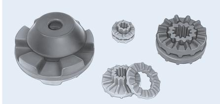
Barry Ring & Bushing Isolators consist of an elastomeric ring and elastomeric bushing and are designed to be directly incorporated into the structural components of the equipment to be mounted. Any number of these isolators can be installed in parallel for greater load capacity and may be stacked in series when greater deflection capacity is required.
