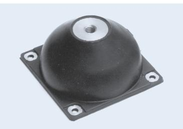
Barry TT-B Mounts are mid-frequency isolators with a large deflection capacity, designed to give both shock and vibration isolation protection. The standard Neoprene version is for applications where temperature extremes are not a factor.
