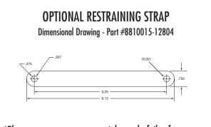
\*Please note, mounts are not inherently fail-safe. They may require the use of a suitable restraining device.
